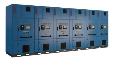
Switchboard to be floor standing with hinged door and hand-rail in front and fixed panel aft. The switchboard is based on a common DC - bus system where power is feed to/from switchboard through power modules. The switchboard system consists of two separate DC busbars within the same cabinet.
