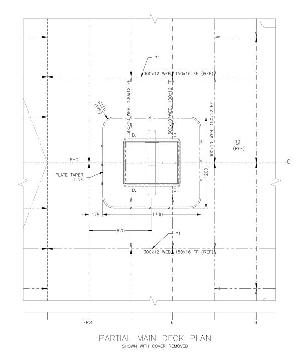
NOTE \*1 OPENING TO BE PROVIDED IN GIRDERS TO FACILITATE SPINDLE REMOVAL.
